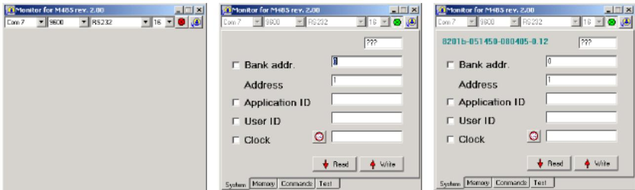
The M485 server in the DelphiStamp communicates using the M485 protocol. This protocol allows for up to 65000 devices. Each device is identified by an address and bank number, both ranging from 0 .. 255. Each device will respond to bank = 0 and address = 1.
