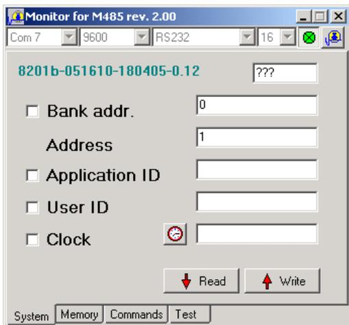
Pressing the Read button will present the DelphiStamp hardware identifier. It contains its serial number, manufacturing date and software revision number.
