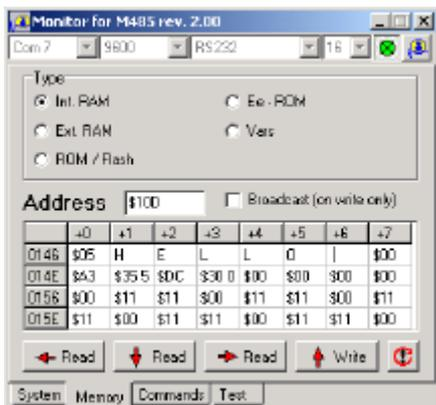
Write in field LcdStr1 of internal RAM at address \$10D the string 'HELLO' starting with the value \$85 on address \$10D. This byte includes a write request on bit 7 and a string length of 5 characters. Press the write button to write it into the DelphiStamp.
