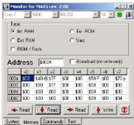
Register DDRC reads \$C0 = %11000000 (\$ is the prefix for Hexa decimal and % for binary numbers), the most left bit, representing DDRC.7 always reads High, meaning this I/O wire is programmed as output.
